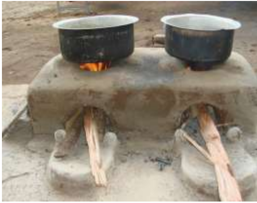
Low cost mud stove for households constructed using clay soil
