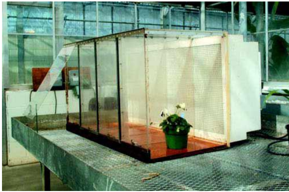
Fig 1. Negative pressure bench-top Traynor et al., 2001
