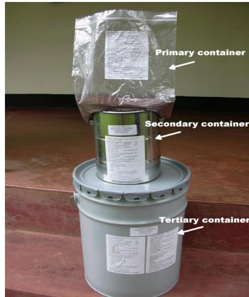
Figure 2: Primary, secondary and tertiary containers used to packaging GMOs
