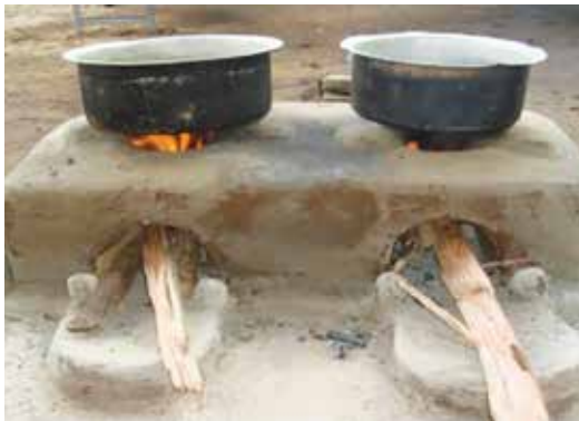
Efficient cooking stoves which utilize few pieces of fire wood for cooking
