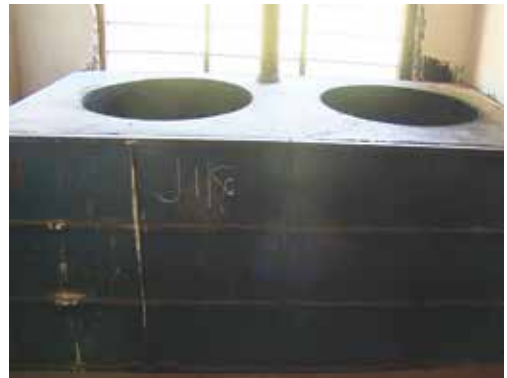
Efficient cooking stoves which utilize wood briquettes for cooking at Chisenga Secondary School
